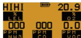
Display in alarm conditions
